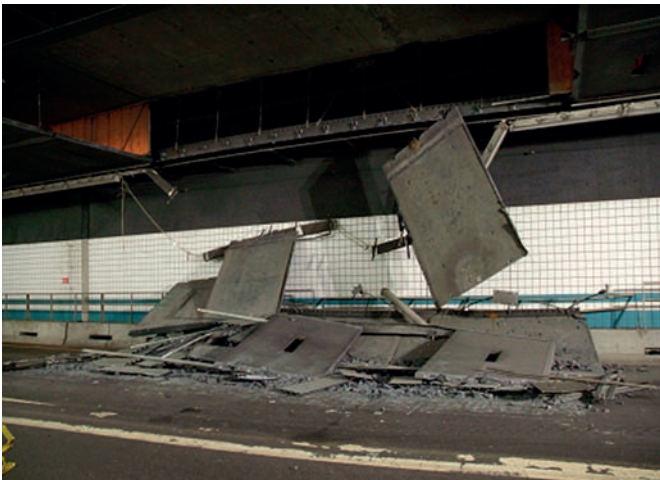
← Figure 2 Approximately 24t of concrete ceiling panels crush a vehicle resulting in a fatality
